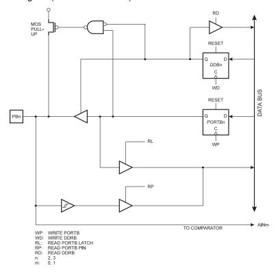
Figure 48. Port B Schematic Diagram (Pin PB4)
