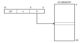
Operand address is contained in 6 bits of the instruction word. n is the destination or source register address.
