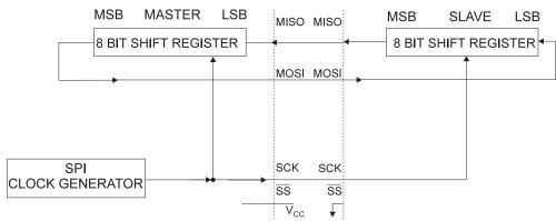
The system is single buffered in the transmit direction and double buffered in the receive direction. This means that characters to be transmitted cannot be written to the SPI Data Register before the entire shift cycle is completed. When receiving data, however, a received character must be read from the SPI Data Register before the next character has been completely shifted in. Otherwise, the first character is lost.
