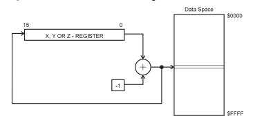
The X, Y or the Z-register is decremented before the operation. Operand address is the decremented contents of the X, Y or the Z-register.
