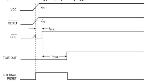
Figure 27. MCU Start-Up, RESET Tied to V<sub>CC</sub>. Slowly Rising V<sub>CC</sub>
