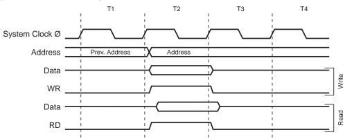
The external data SRAM access is performed in two System Clock cycles as described in Figure 22.
