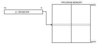
Program execution continues at address contained by the Z-register (i.e. the PC is loaded with the contents of the Z-register).
