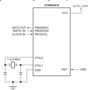
When writing serial data to the AT90S4414, data is clocked on the rising edge of CLK.
