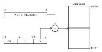
Operand address is the result of the Y or Z-register contents added to the address contained in 6 bits of the instruction word.
