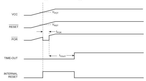
Figure 28. MCU Start-Up, RESET Controlled Externally
