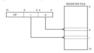
**Figure 10.** Direct Register Addressing, Two Registers Operands are contained in register r (Rr) and d (Rd). The result is stored in register d (Rd).
