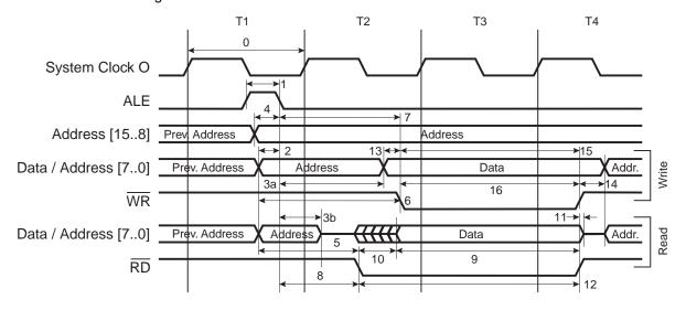
Note: Clock cycle T3 is only present when external SRAM waitstate is enabled
