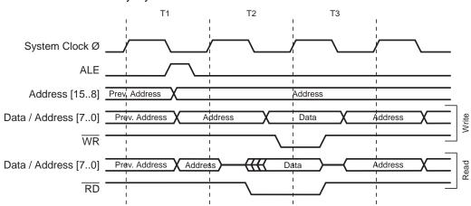
The external data SRAM memory access cycle with the Wait State bit enabled (Wait State active) is shown in Figure 24.
