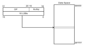
A 16-bit Data Address is contained in the 16 LSBs of a two-word instruction. Rd/Rr specify the destination or source register.
