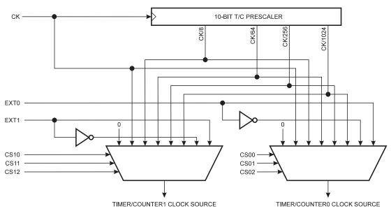
For Timer/Counters 0 and 1, the four different prescaled selections are: CK/8, CK/64, CK/256 and CK/1024, where CK is the oscillator clock. For the two Timer/Counters 0 and
