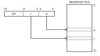
Operands are contained in register r (Rr) and d (Rd). The result is stored in register d (Rd).
