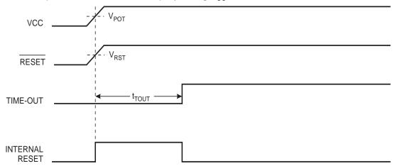
Figure 24. MCU Start-Up, RESET Tied to VCC. Slowly Rising V<sub>CC</sub>
