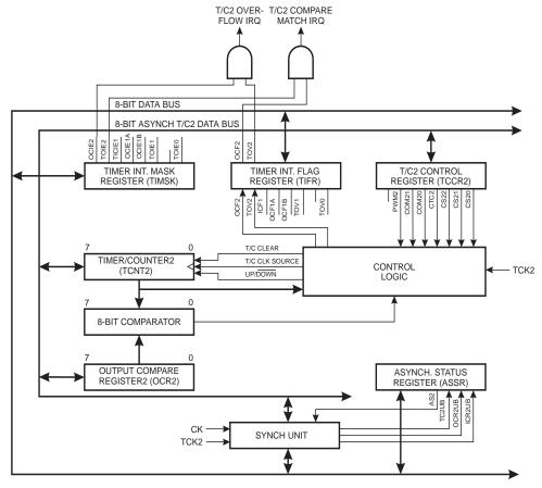
The 8-bit Timer/Counter2 can select clock source from TCK2 or prescaled TCK2. It can also be stopped as described in the specification for the Timer/Counter Control Register TCCR2.
