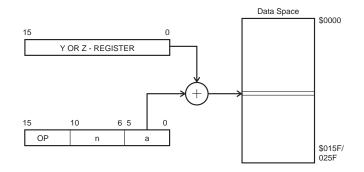
Operand address is the result of the Y or Z-register contents added to the address contained in 6 bits of the instruction word.
