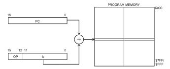
Program execution continues at address PC + k + 1. The relative address k is from -2048 to 2047.
