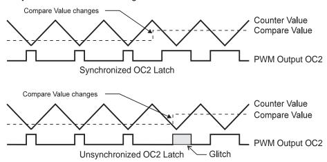
During the time between the write and the latch operation, a read from OCR1A or OCR1B will read the contents of the temporary location. This means that the most recently written value always will read out of OCR1A/B.
