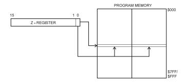
Constant byte address is specified by the Z-register contents. The 15 MSBs select word address (0 - 2K/4K) and LSB, select low byte if cleared (LSB = 0) or high byte if set (LSB = 1).
