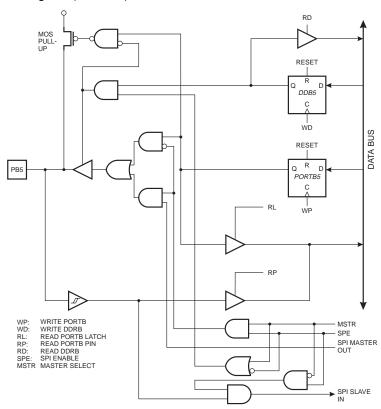
Figure 52. PORTB Schematic Diagram (Pin PB6)
