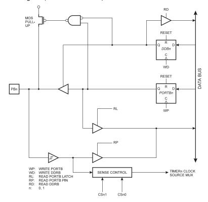
Figure 49. PORTB Schematic Diagram (Pins PB2 and PB3)
