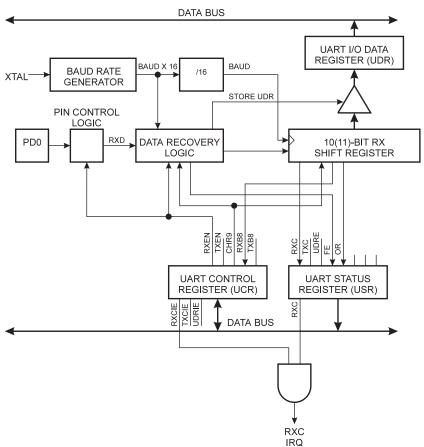
The receiver front-end logic samples the signal on the RXD pin at a frequency 16 times the baud rate. While the line is idle, one single sample of logical zero will be interpreted as
