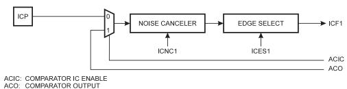
If the noise canceler function is enabled, the actual trigger condition for the capture event is monitored over 4 samples before the capture is activated. The input pin signal is sampled at XTAL clock frequency.
