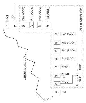
Note that since  $AV_{CC}$  feeds the Part A output drivers, the RC network shown should not be employed if any Port A serve as outputs.
