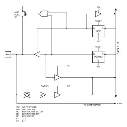
Figure 50. PORTB Schematic Diagram (Pin PB4)
