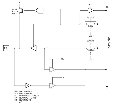
Figure 55. PORTC Schematic Diagram (Pins PC6)
