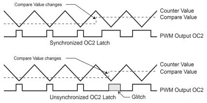
During the time between the write and the latch operation, a read from OCR2 will read the contents of the temporary location. This means that the most recently written value always will read out of OCR2.
