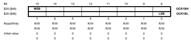
The output compare registers are 16-bit read/write registers.
