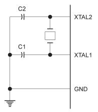
Figure 2. External Clock Drive Configuration
