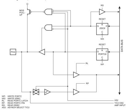
Figure 56. PORTC Schematic Diagram (Pins PC7)
