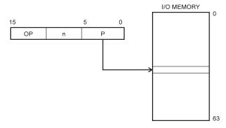
Operand address is contained in 6 bits of the instruction word. n is the destination or source register address.
