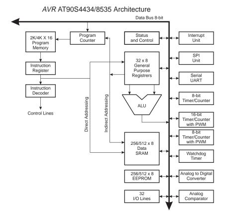
The ALU supports arithmetic and logic functions between registers or between a constant and a register. Single register operations are also executed in the ALU. Figure 3 shows the AT90S4434/8535 AVR Enhanced RISC microcontroller architecture.
