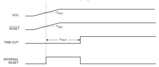
Figure 25. MCU Start-Up, RESET Controlled Externally
