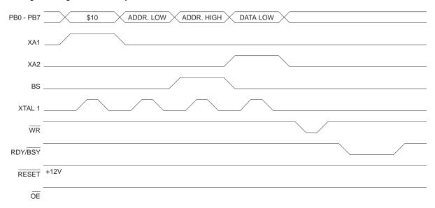
Figure 65. Programming Flash High Byte
