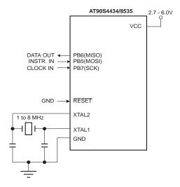
When writing serial data to the AT90S4434/8535, data is clocked on the rising edge of SCK.
