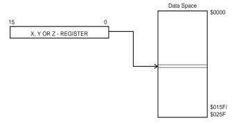
Operand address is the contents of the X, Y or the Z-register.
