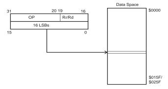
A 16-bit Data Address is contained in the 16 LSBs of a two-word instruction. Rd/Rr specify the destination or source register.
