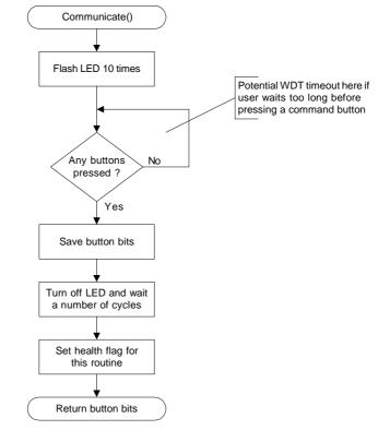
If a command button is pressed in time, the routine sets its health flag and returns the button press bit pattern.
