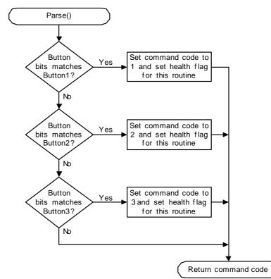
Note that if two or more command buttons are pressed simultaneously, the parser will never find a match and its health flag is never set. Because if this, the health check in the main loop will not reset the WDT, and a system reset could occur if the main loop is not executed successfully and quickly enough a second time. This is an example showing that unexpected inputs may cause problems if not handled by a default case in the switch block.
