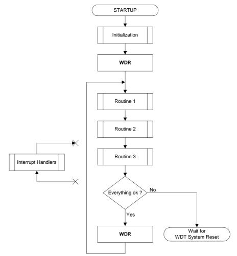
Note that if the timeout period is chosen very tight, an unusual number of interrupts could cause a WDT System Reset. This must be taken into consideration when choosing the timeout period.
