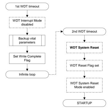
The Write Complete Flag could be a byte in EEPROM indicating whether the backup operation was finished before the system reset. This flag is checked in the startup code if the WDT Reset Flag is set, and the backed up parameters can be used for restoring system state or debugging purposes. The flag should be cleared during initialization to invalidate the parameters if other types of resets occur.
