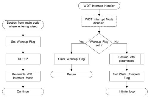
Note that the wakeup flag must be set manually prior to entering sleep mode to ensure that the correct part of the handler is executed on wakeup. The WDT Interrupt Mode must be re-enabled outside the interrupt handler after serving the wakeup interrupt.
