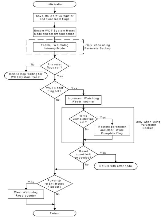
The first conditional branch handles the case where no reset flags are set upon startup. Since the reset flags are always cleared in the initialization routine, this only happens when runaway code wraps back to address 0 and runs the startup code once again without a reset. This clearly indicates a bug or fault in software and is handled like a WDT System Reset. The initialization routine just enters an infinite loop and waits for the WDT to reset the device properly.
