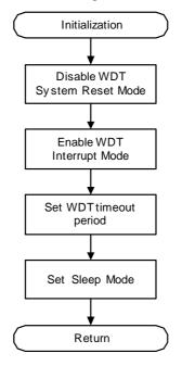
The main loop of this example flashes the LED connected to PB0 10 times to show that it is awake. It then resets the WDT, enables the WDT Interrupt Mode and enters sleep mode. When the WDT times out, it wakes up the CPU again. The interrupt handler disables WDT Interrupt Mode, so that no unneccessary interrupts are generated if the main loop runs long before entering sleep mode once again.
