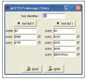
When finished setting the mask and filters, the MCP2515 can be written by pressing the "Write" button while in "Configuration" mode.
