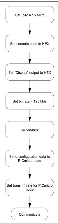
Must set the on-board oscillator value so the bit timing will be calculated properly. (Options > MCP2515)
