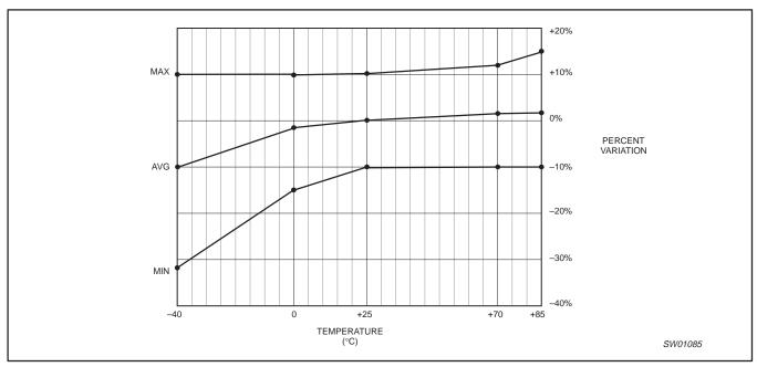
Figure 13. Typical frequency variation over process at  $V_{DD}$  = 2.3 V to 3.0 V
