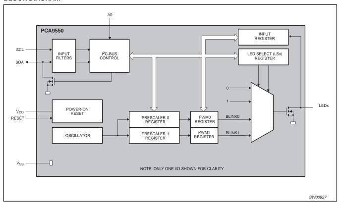
Figure 2. Block diagram
