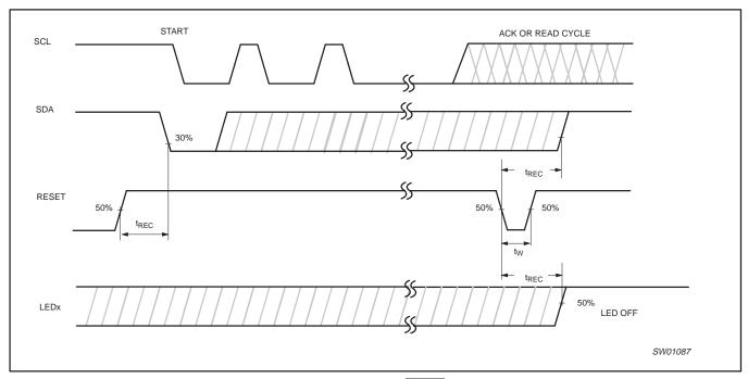
Figure 15. Definition of RESET timing
