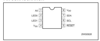
Figure 1. Pin configuration
