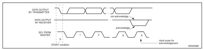
Figure 8. Acknowledgement on the I<sup>2</sup>C-bus
