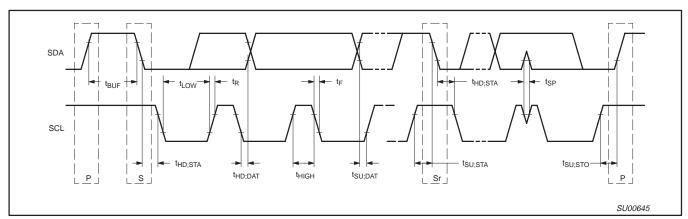
Figure 16. Definition of timing
