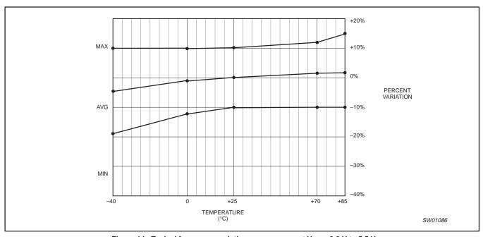
Figure 14. Typical frequency variation over process at  $V_{DD}$  = 3.0 V to 5.5 V
