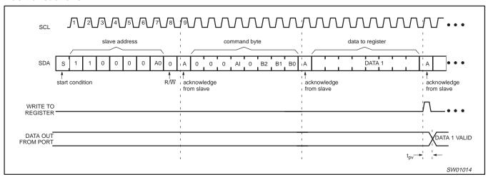
Figure 9. WRITE to register
