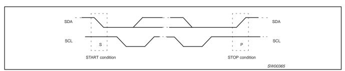
Figure 6. Definition of start and stop conditions
