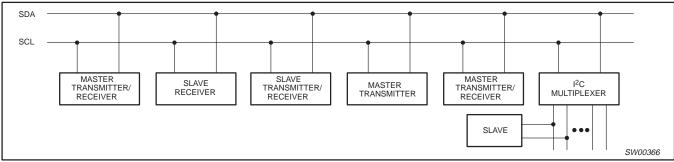
Figure 7. System configuration
