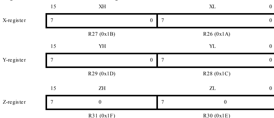
Figure 10-3. The X-, Y- and Z-Registers
