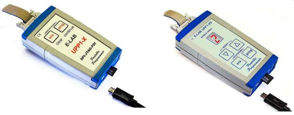
Standalone operated with SD card or PC. With internal battery with 3.7V/700mAh
