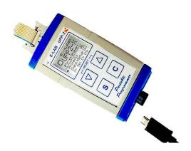
Standalone operated with microSD flash card Upto 63 projects stored on the card are usable. Elegant and easy user interface Completely controllable by the PC. Internal battery with 3.7V/700mAh
