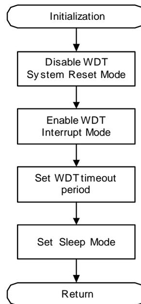
The main loop of this example flashes the LED connected to PB0 10 times to show that it is awake. It then resets the WDT, enables the WDT Interrupt Mode and enters sleep mode. When the WDT times out, it wakes up the CPU again. The interrupt handler disables WDT Interrupt Mode, so that no unnecessary interrupts are generated if the main loop runs long before entering sleep mode once again.
