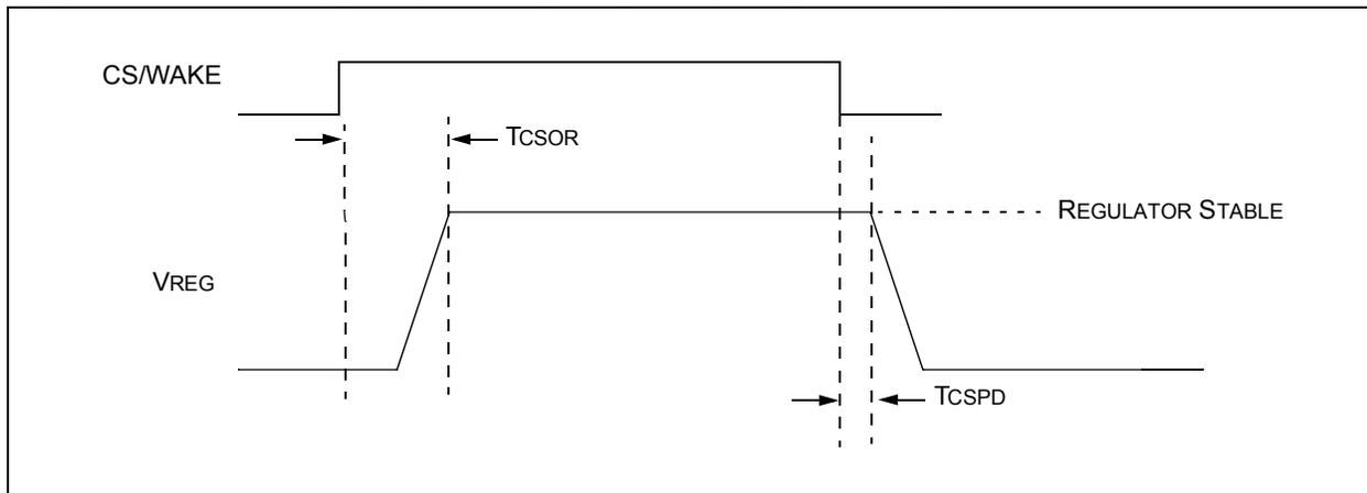
**FIGURE 2-3: REGULATOR TIMING DIAGRAM ON BUS ACTIVITY**
