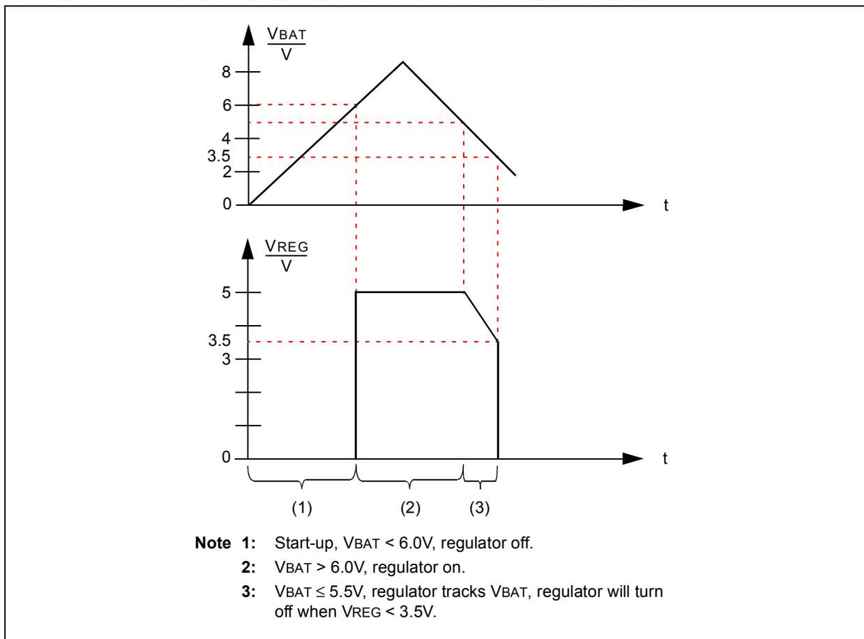
**FIGURE 1-5: VOLTAGE REGULATOR OUTPUT ON POWER DIP**
