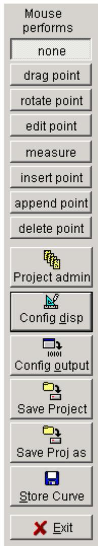
The upper half of the picture at left shows the properties which can be chosen for mouse clicks and mouse moves.
