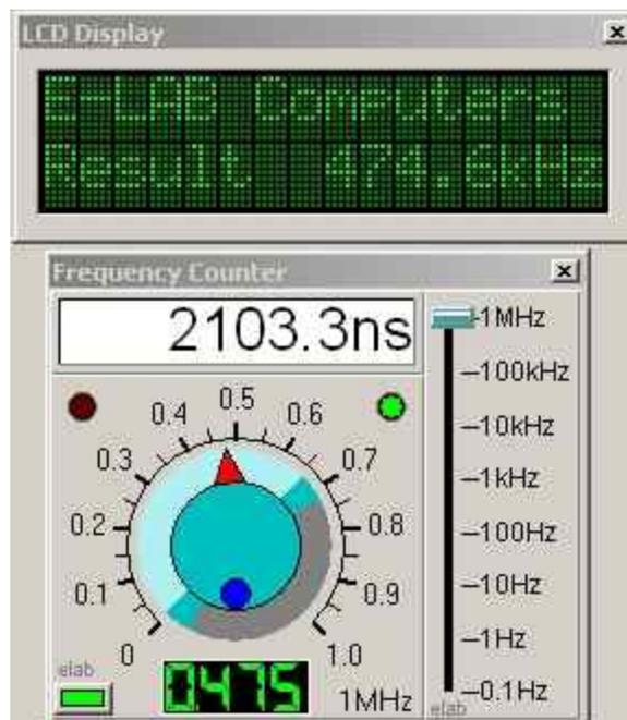
With the slide switch on the right you select a frequency range 0...0,1Hz, 0...1Hz, etc. up to 0...1MHz. The poti is used to select the frequency. The small button on the lower left corner starts / stops the frequency counter.
