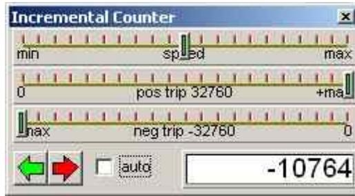
The green/red arrows are used to control the actual value ("turn the encoder"). The driver uses the interrupt so changes are only possible in "Run" mode.
