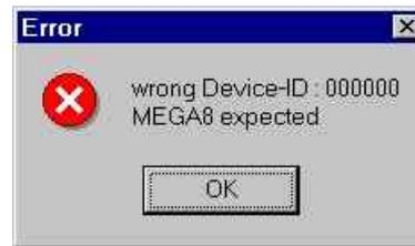
the controller fuses are (already) wrong and you need to apply the correct clock source to re-program the chip. There is no information what kind of clock source is "correct".
