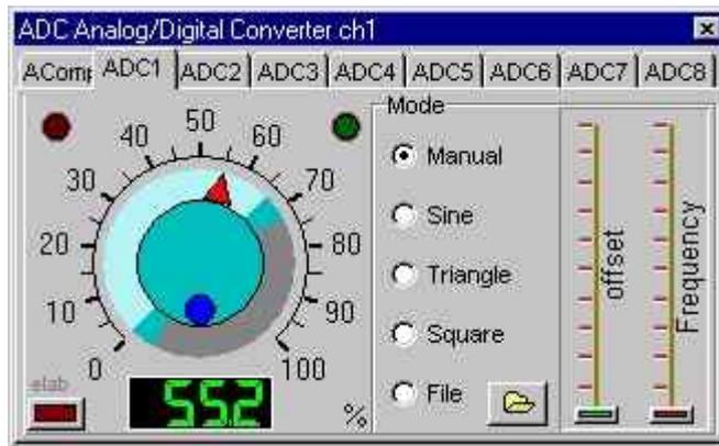
Controllers with 10 bit ADC have 2 result bytes. By default the result is right adjusted (the high byte contains only the 2 most significant bits). Only this mode is supported by the simulator.
