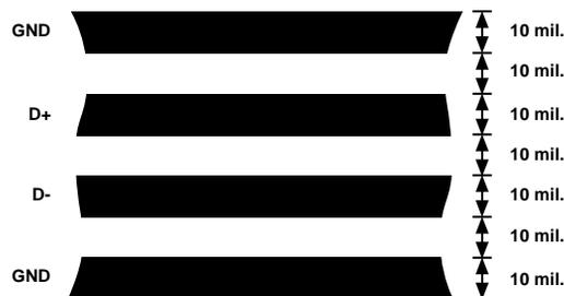
Figure 14. Arrangement of Signal Tracks
