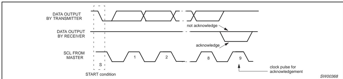
Figure 8. Acknowledgement on the I<sup>2</sup>C-bus
