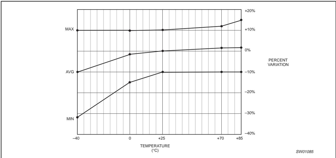
Figure 13. Typical frequency variation over process at V<sub>DD</sub> = 2.3 V to 3.0 V
