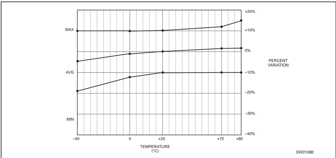
Figure 14. Typical frequency variation over process at V<sub>DD</sub> = 3.0 V to 5.5 V
