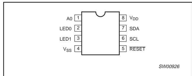
Figure 1. Pin configuration
