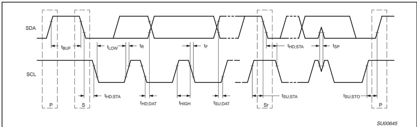
Figure 16. Definition of timing
