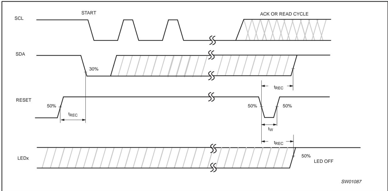
Figure 15. Definition of RESET timing
