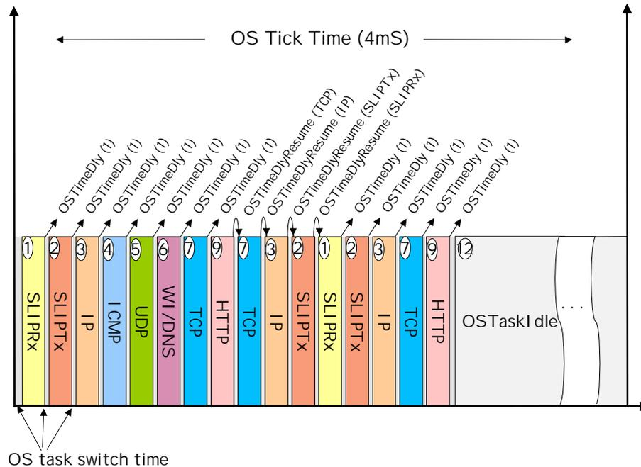
Figure 5. Protocol Task flow (typical HTTP request)
