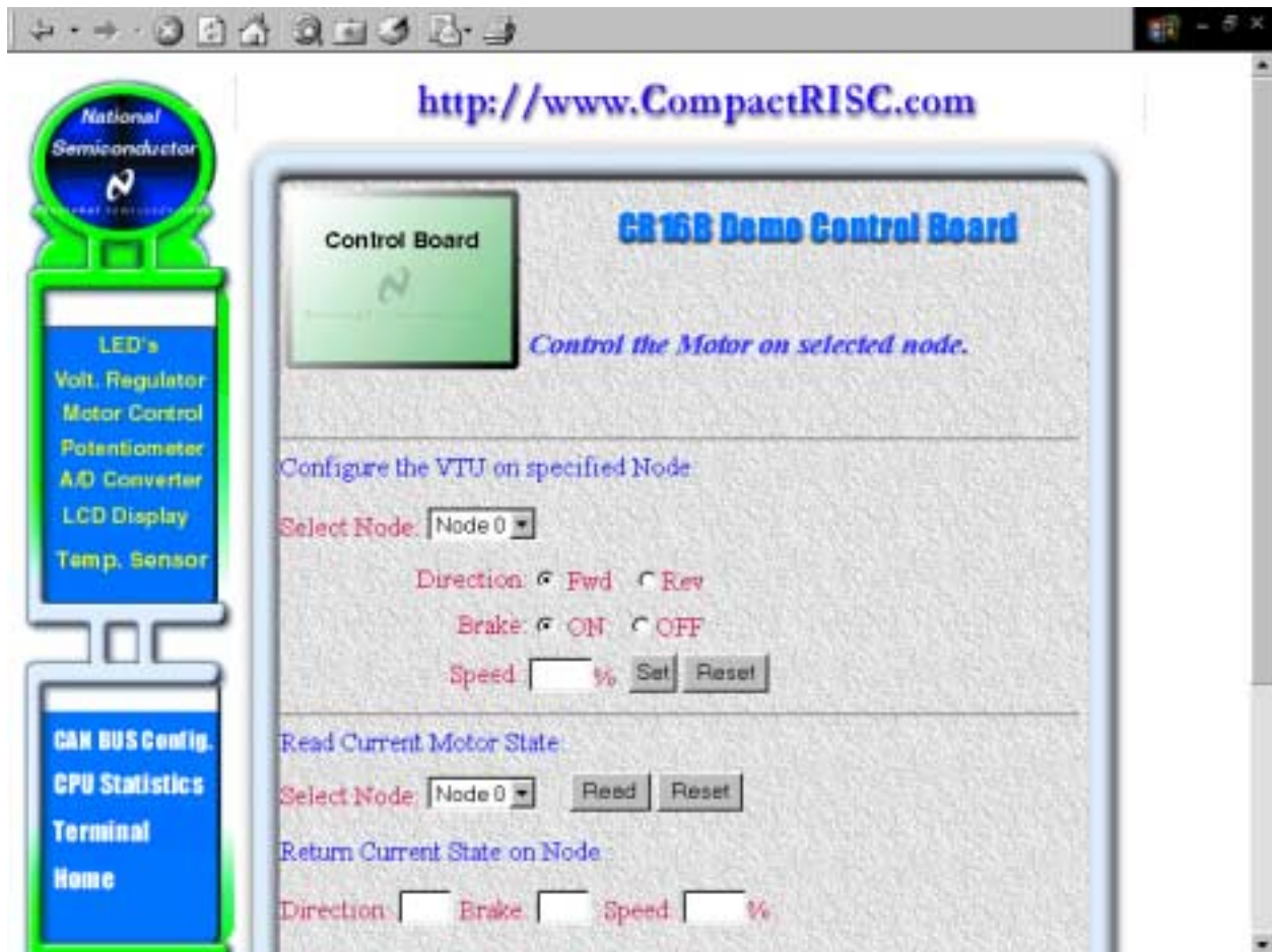
Figure 25. An Embedded Motor Control Page from the Project
