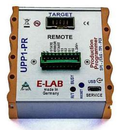
With the build-in remote interface the UPP1-PR becomes remote controlable. By 4 control lines one out of 16 projects stored on the flash card can be selected.
