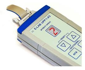
Standalone operated with SD card or PC. With internal battery with 3.7V/700mAh
