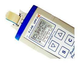
Standalone operated with microSD flash card Upto 63 projects stored on the card are usable. Elegant and easy user interface Completely controllable by the PC. Internal battery with 3.7V/700mAh
