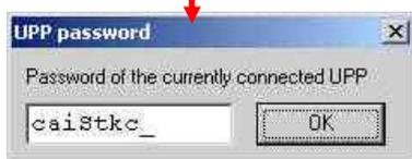
If an additional or new key for the encryption of a UPP1-X project is needed this key/password of a connected UPP1-X programmer can be readout with the menu item above. The user of this programmer then passes this key to the project and file owner. The latter now must add this password/key in the dialog list below.
