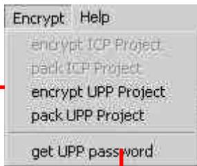
The content of an encrypted file is scrambled and only readable with a unique key. This key programmed and fixed in the UPP1-X programmer. Each device has its own unique key. So files which are encrypted with this key can only be read by this device.
