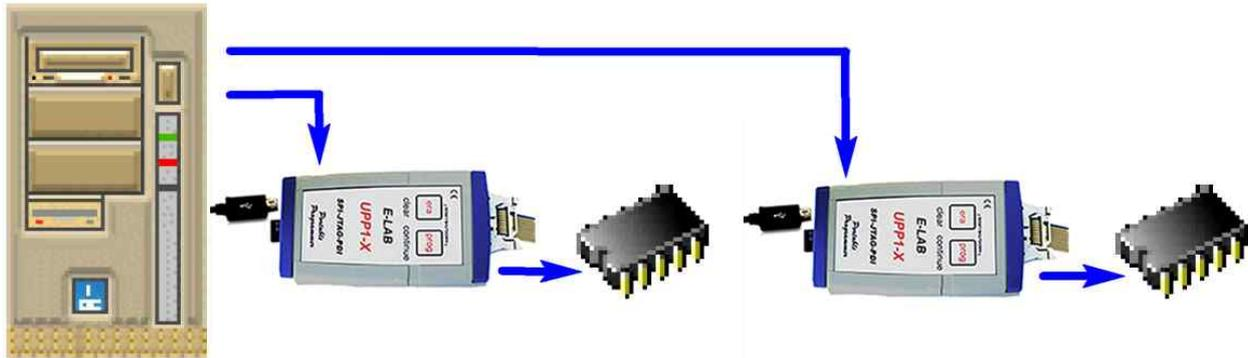
With mass production of electronic boards build with Single-Chips there is often the problem how to program the CPUs within the automatic testing of the board. Common ISP programmers are cheap and often easy to use but they can't be easily integrated into the automatic test environment.
